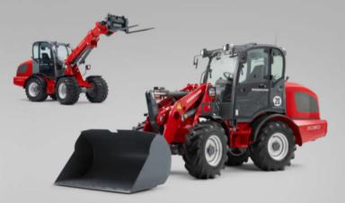
**Powerful wheel loaders.** Optionally with load arm or telescopic arm.
