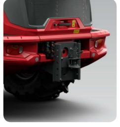
**Flexible trailer operation up to 18 tonnes.** A self-recovering hitch is standard. Optionally, an automatic trailer hitch is on offer. In addition, the following hitch options in conjunction with a height-adjustable hitch block are available: Automatic trailer hitch, K50 ball hitch (private car trailers), K80 ball hitch, piton fix and CUNA D3. To move trailer loads safely, there are both a dual line compressed air brake and a hydraulic trailer brake.
