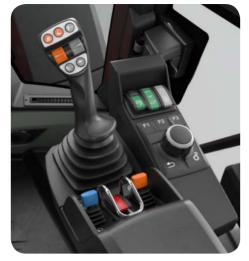
**Hydraulic oil volume adjustment.** If necessary, the "Jog Dial" control element can set the hydraulic oil flow manually. This is advantageous if the machine is driving a hydraulic attachment which does not need the machine's full hydraulic performance. In this way, the operator can work very delicately and in a resource-friendly manner with machine and attachment.
